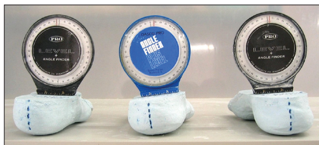
Figure 6: Forefoot eversion or inversion position differs significantly between the three cast techniques
