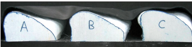
Figure 12: Cross section at mid-arch. Note steepness of slope in suspension cast A
